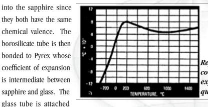
The uncommon behavior of the coefficient of expansion of fused quartz gives rise to special problems in dealing with it. The figure shows the rapid drop to zero expansion near room temperature and the negative expansion values at lower temperatures. This is a rare phenomenon associated with materials that have strong covalently bonded chains (like Si-O2) and much weaker bonds between the chains. Consider a string of atoms connected by strong bonds and weakly connected with neighboring chains. As
